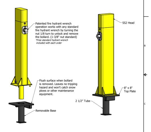
56 lbs 9 lbs 11/2/2009 PROPRIETARY AND CONFIDENTIAL THIS DRAWING CONTAINS PROPRIETARY INFORMATION OF BLUE EMBER TECHNOLOGIES, LLC. ANY USE OF THIS DRAWING OR THE
